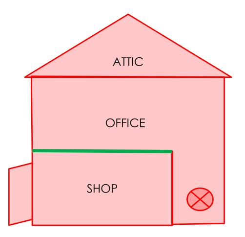
Test 2: 6.4 achr @50 PA Biggest leaks through roof
