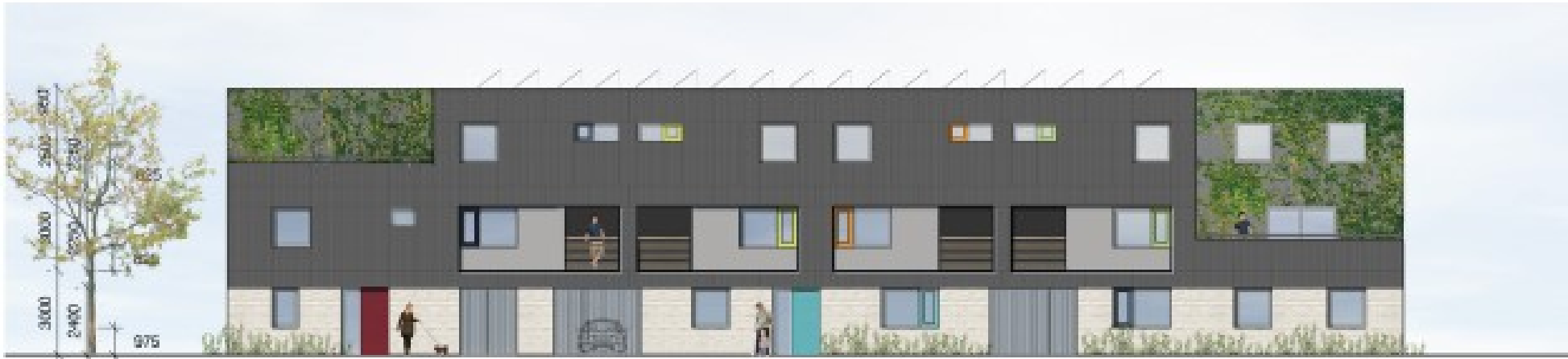
EAST ELEVATION - 35% glazing target
