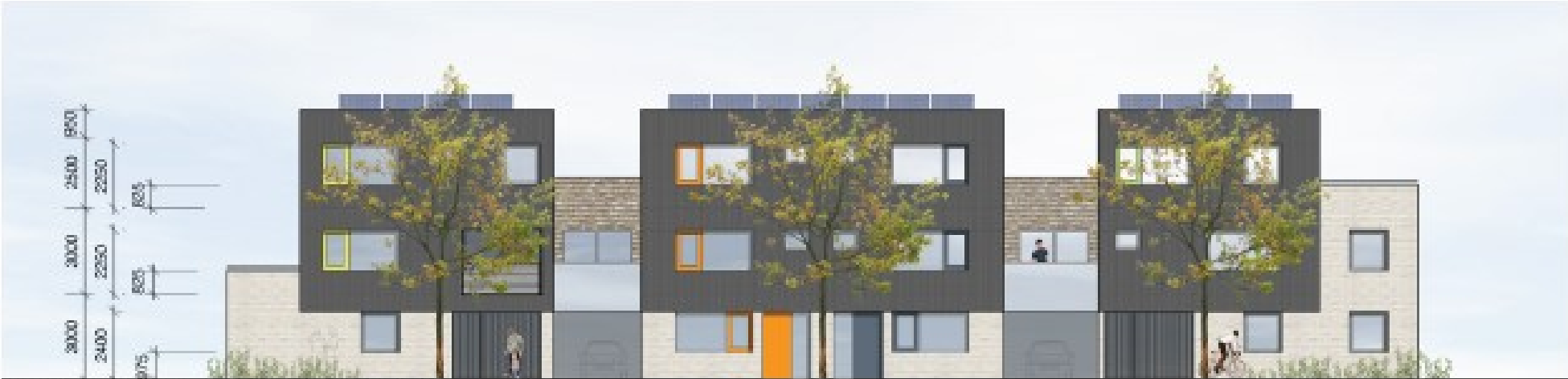
SOUTH ELEVATION - 40%-45% glazing target - external blinds
