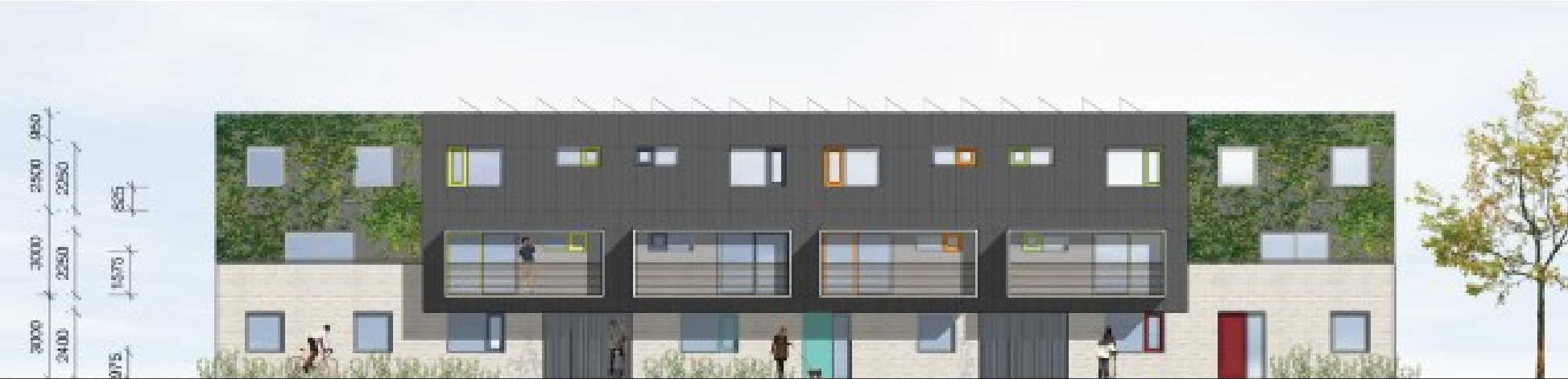
WEST ELEVATION - 30% glazing target - external blinds
