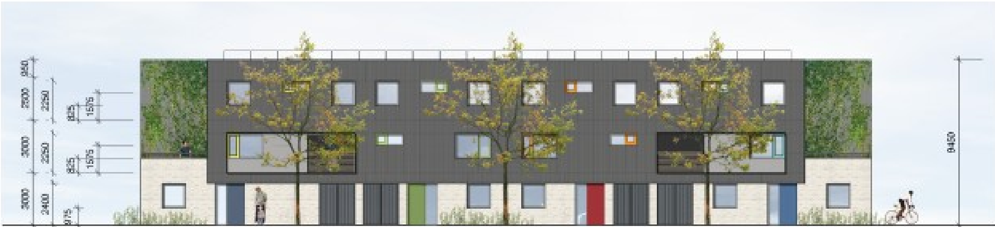
NORTH ELEVATION - 20-25% glazing target - no shading
