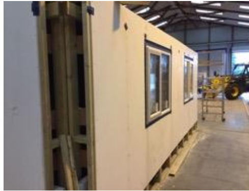
Offsite – Large Panel
