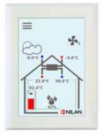
The Compact P is controlled using its CTS 602 HMI touch panel, featuring a wide range of functions, e.g., menu-controlled operation, weekly programme settings, filter monitor with timer, fan speed adjustment, summer bypass, supply-heating element control, error messages etc.
